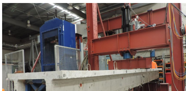
Figure 1: Experimental arrangement for the simply supported box-girder bridge model [2].
