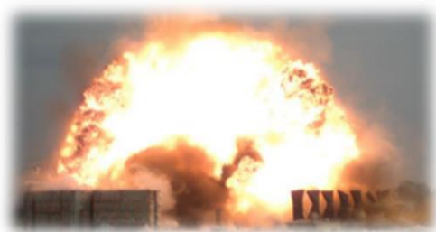
Warhead detonation during arena trial
